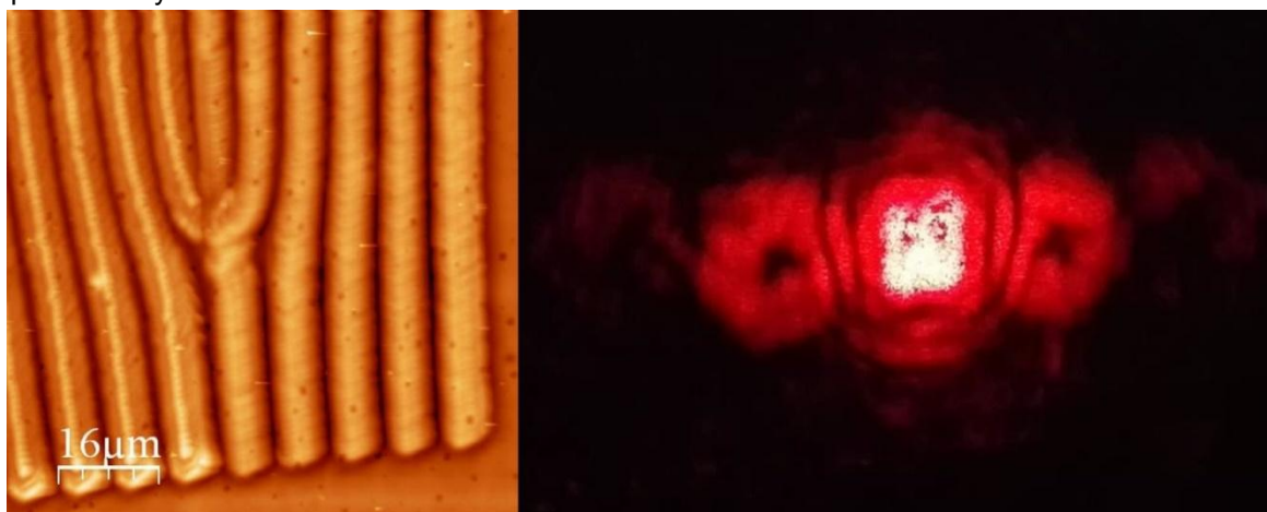
Figure 1. AFM image of forking relief grating in azo-polymer and light diffraction on it generating Laguerre-Gauss vortex beams.
